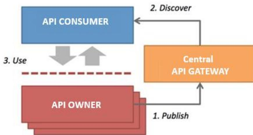
**Figure 3. Roles of API-driven Integrated Applications**
